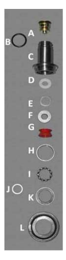
REBUILDING POT BEARING HOUSINGS: The used assembly is disassembled, cleaned and inspected. Epic **always** replaces the felt sealing washer (D), upper needle bearing (F), nylon spacer bushing (G), lower outer race (H), and bearing cage, polyamide (I). Any static parts that show wear or faults are also replaced. The rebuilt assembly is lubricated with Kluber synthetic grease.
